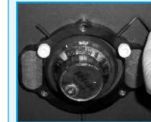
Tighten set screws snug to the dial ring
