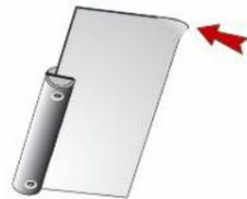
Bend one of the corners of the Door Latch Opening Card, so it will fit more easily between door and door frame.
