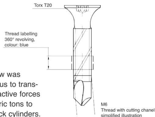
This Pull Screw was developed by us to transfer extreme tractive forces of up to 5 metric tons to high quality lock cylinders.
