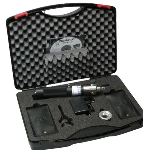
Our battery operated electric Pick Gun uses the percussion principle. The necessary vibration frequency and strength of the pick is delivered by an eccentric. Therefore easy picking of multi-pin pin and disc tumbler locks is possible.
