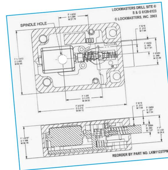
Provide an accurate, x-ray type view of the lock. Each template is reproduced in actual size, front and top view and the spindle hole is pre-drilled for easy installation. The Magnetic Drill Sites are reusable, heavy-duty coated vinyl with magnetic backs.
