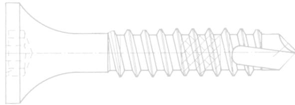
A colour marking of approx. 10 mm on the first threads shows an unused screw.
