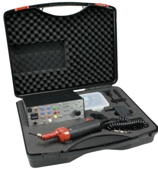
The Multipick-System works with a special pick blade – inserted in the Multipick’s blade holder – which is entered into the keyway.
