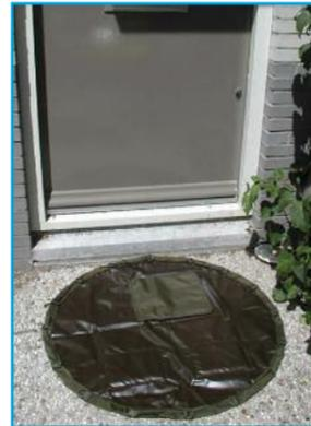
The mat is placed on the floor and the tools can be spread out on the work surface. The round mat has a rope around its outside and in case of a disturbance the mat will fold like a bag by pulling on the rope. All tools which are placed on the mat are inside the bag now. The working mat has a separate part which can be unfolded.
