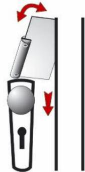
Pull the door handle with one hand and use the other hand to insert the Door Latch Opening Card with back and forth movements between door and door frame.
