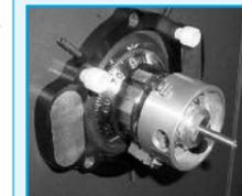
Using the Chuck Key, adjust the Gripper Set to fit around the dial
