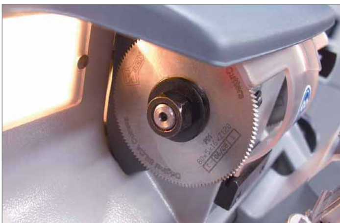
Prismatic cutter made of HSS
